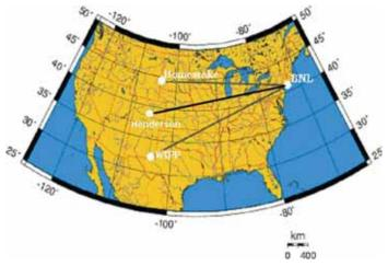
**Fig. 1:** Possible extra long neutrino baselines from BNL to Lead (Homestake) SD ( $\Box$  2540 Km), to Carlsbad (WIPP) NM ( $\Box$  2900 km), and to the Henderson Mine in Colorado ( $\Box$  2700 km).
