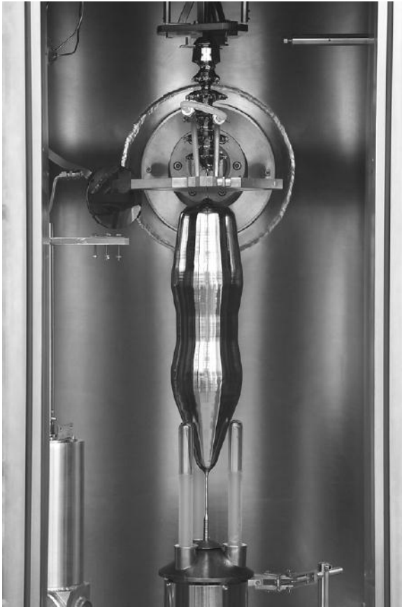
5kg ^{28}\text{Si} crystal grown by the float zoning method
