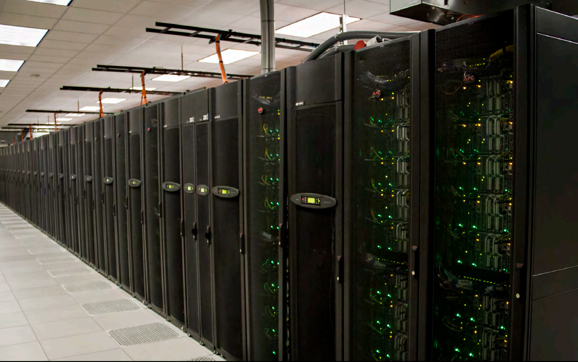
Stampede (Texas Advanced Computer Center) 6,400 Dell C8220 nodes (102,000 cores + 390,000 co-proc cores) 10 Pflops aggregate performance
