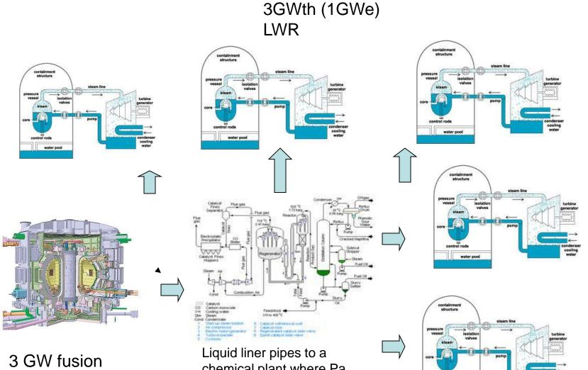
3 GW fusion plant (ITER image) Liquid liner pipes to a chemical plant where Pa is separated and mixed with uranium
