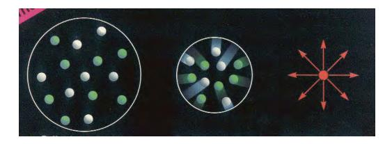
A capsule containing deuterium and tritium is irradiated by x-ray, laser or particle beams, compressing and heating the fuel to ignition
