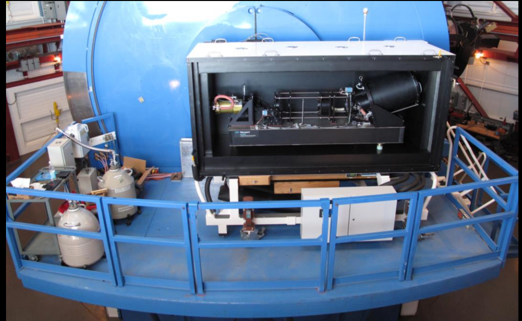
Side insulation panel is removed to show instrument interior
