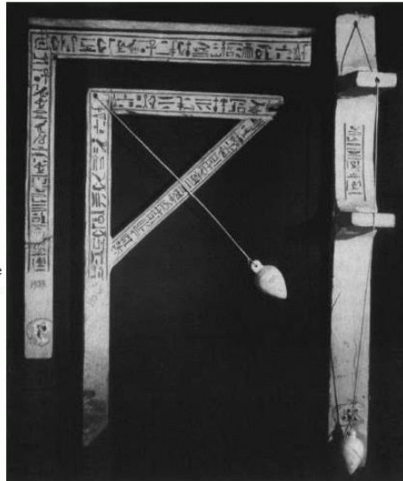
Fig. 6.4 A plumb, a square, and a square level from the tomb of Senedjem at Deir el-Medineh. (Cairo 27280, 27259, 27258)
