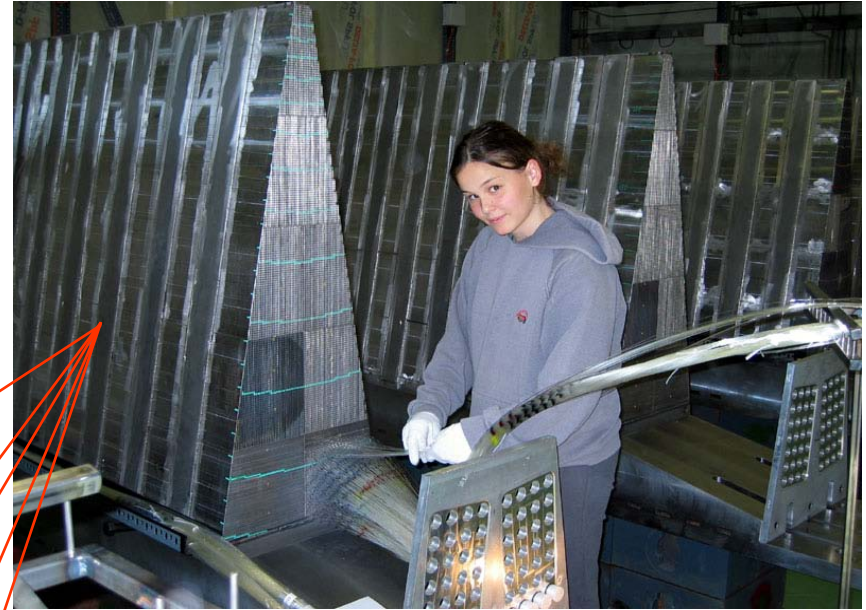
Hungarian student inserting quartz fibres into steel wedges
