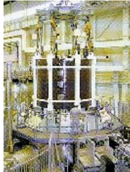
REMOTE MAINTENANCE OF DIVERTOR CASSETTE
