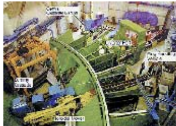
REMOTE MAINTENANCE OF DIVERTOR CASSETTE
