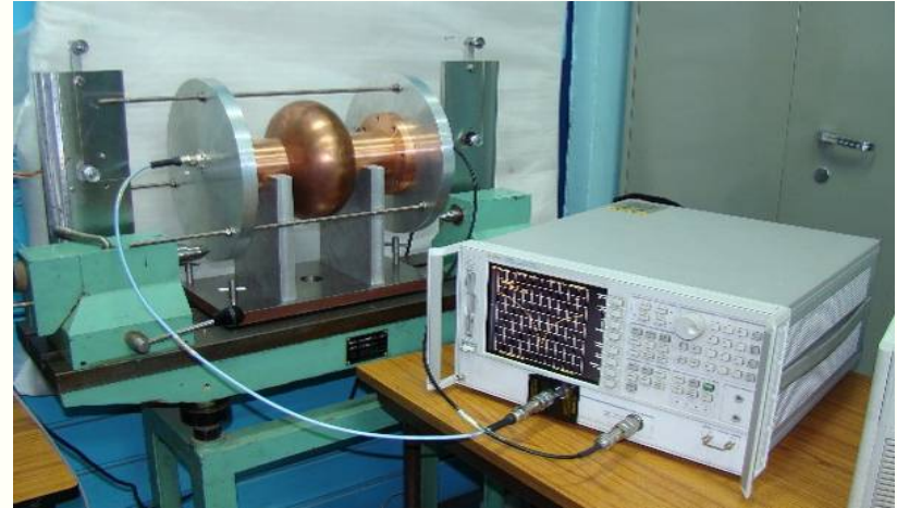
Bead Pull Measurement Setup for Assembled Cavity
