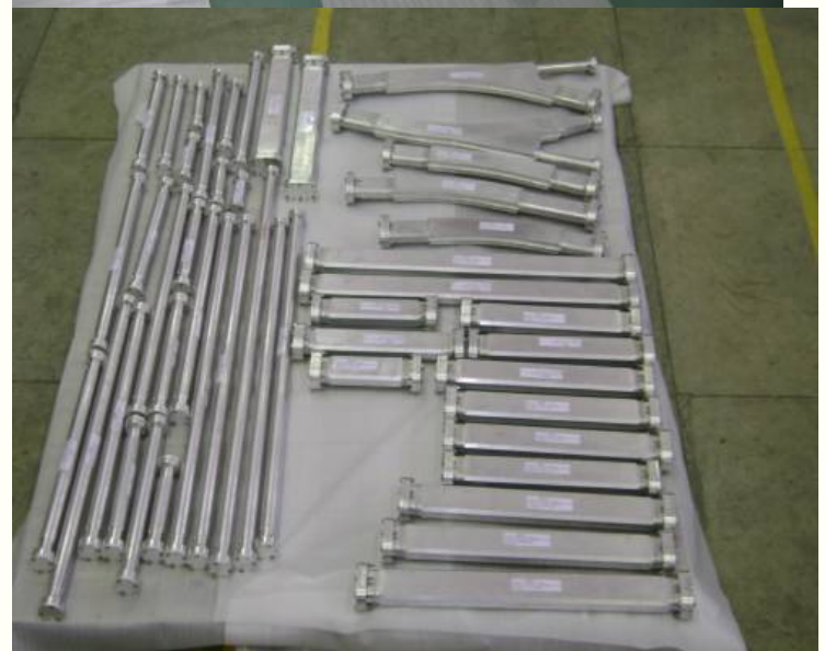
Completed vacuum chambers
