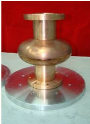
Assembled Cavity with beam pipe & Flanges
