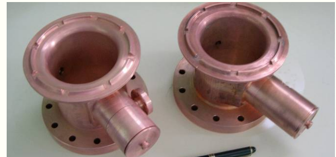
End Group Prototypes made from Cu
