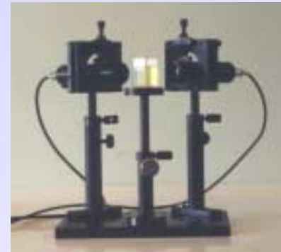
UV-LED Based Fluorimeter with Integrated Lock-in Amplifier (after Prof. Zukauskas, U of V.)
