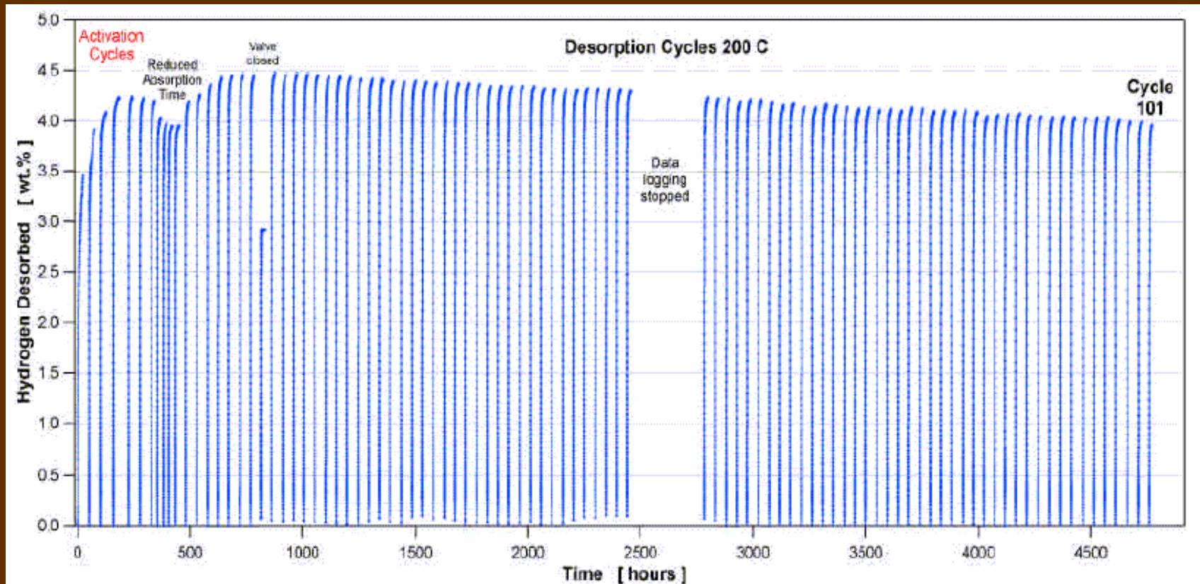
Average capacity loss: 0.005wt% per cycle.
