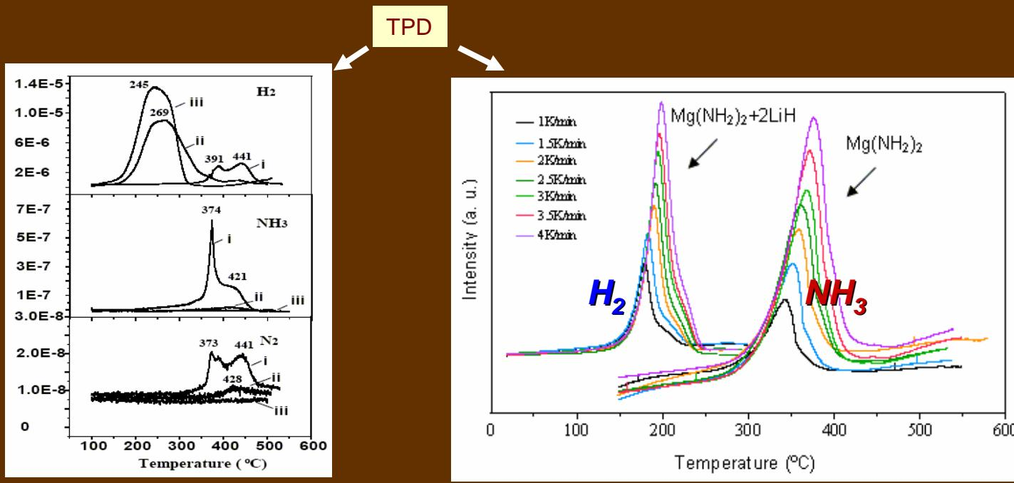
i. Pure  $\text{LiNH}_2$ ; ii.  $\text{LiNH}_2 + \text{LiH}$  (1/1); iii.  $\text{LiNH}_2 + 2\text{LiH}$  (1/2)
