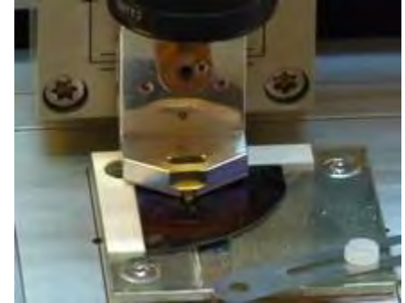
IBM's mechanism works like an atomic force microscope (AFM) but with a heated tip that can sculpt 3D nanometer resolution patterns. (Source: IBM)
