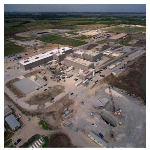
Aerial view of the SSC North Campus in September 1992, showing the Magnet Development Lab (at left) and Magnet Test Lab (center). The long, narrow building at right is where accelerator systems string tests occurred; the shaft at lower right leads down to the Main Ring tunnel, then about to begin construction.
