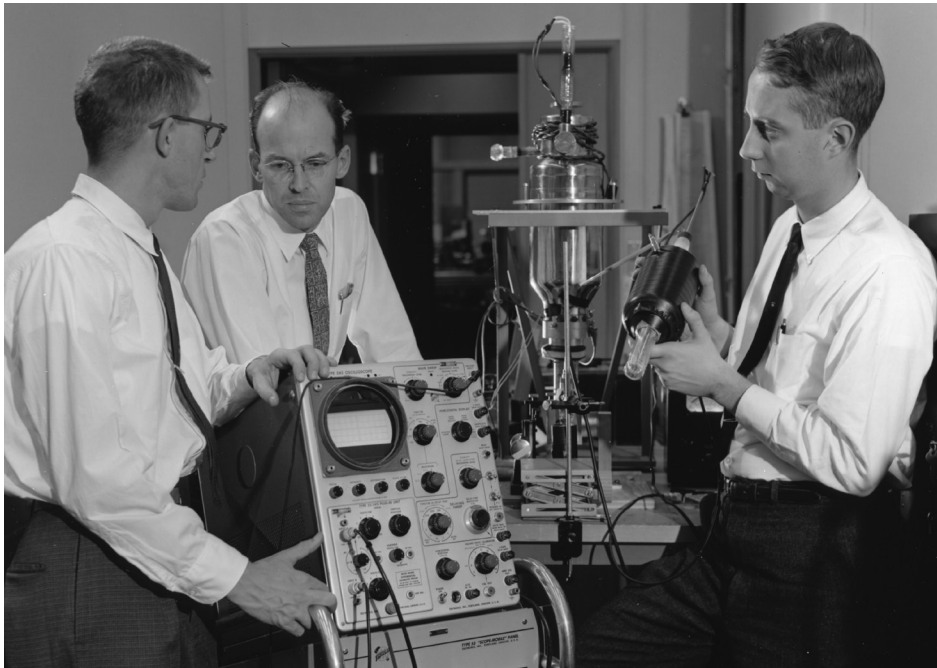
Fig. 8. L-R: Gunther E. Fenner, Robert N. Hall and Jack D. Kingsley, November 1, 1962. Kingsley holds a refrigerated container in which the laser operates at liquid-air temperatures. In the background another laser operates within a container chilled by liquid helium. The oscilloscope makes it possible to observe the shape of pulses produced by the laser. Photo courtesy General Electric Research Laboratories (used by permission), and the AIP Emilio Segre Visual Archives, Hecht Collection.
