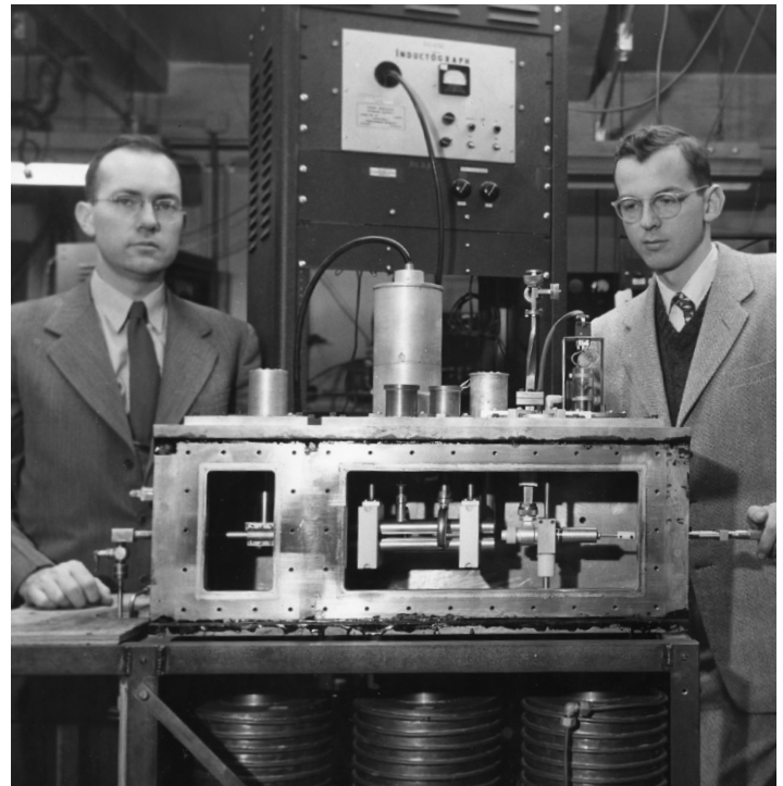
Fig. 1. Charles Townes (left) and J. P. Gordon standing with the second ammonia beam maser at Columbia University, 1955. AIP Emilio Segre Visual Archives, Physics Today Collection.
