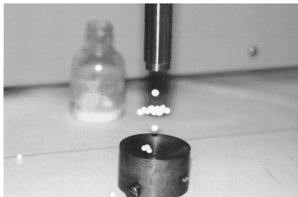
Styrofoam balls levitated in a sound field
