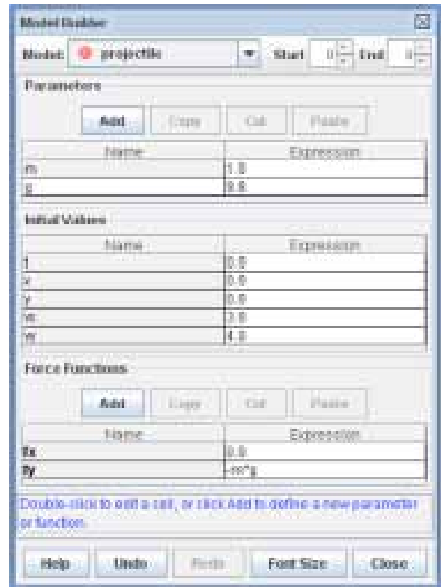
Figure 3: Model Builder with a dynamical model of a simple projectile.
