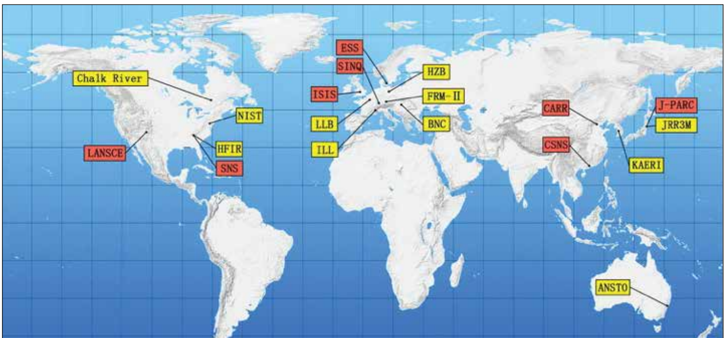
Map of the bigger neutron research centers. Red are sources that produce their neutrons by Spallation, yellow by fission.
