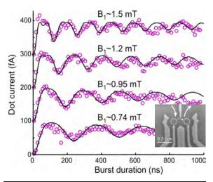
Coherent oscillations of a single electron spin. The current flow (vertical axis) reflects the spin direction, and the spin rotation angle is controlled by the duration of the oscillating field burst (with amplitude B1). Curves offset for clarity. Inset: scanning-electron-microscope image of metallic gates on top of a two-dimensional electron gas. Quantum dots (indicated by white dotted circles) are formed by applying negative voltages to the gates.
