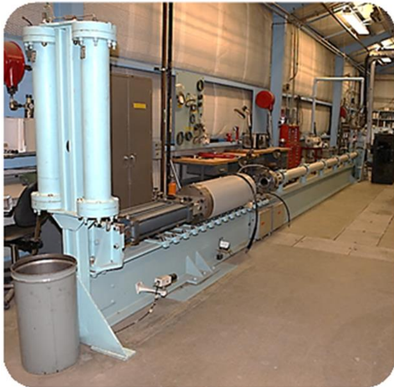
Figure 3. Single-stage light gas gun at STAR, a Sandia facility for shock physics experiments. Laboratory test launchers at STAR can test nearly any type of material (explosives, chemical and biological simulants, ceramics, powders). We recently celebrated its first gas gun-driven impact test, which occurred on September 19, 1969. (Image credit – Sandia National Laboratories)
