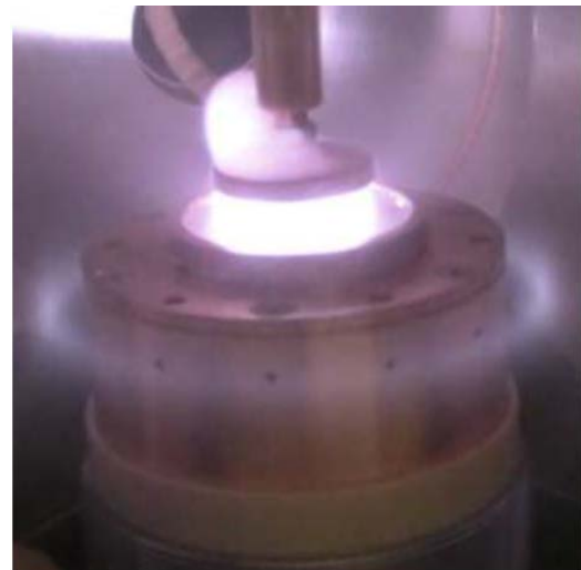
Figure 1: Laboratory test of a liquid-metal cathode. (Photo courtesy of General Electric.)
