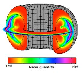
A computer simulation (with the NIMROD code) of neon injected uniformly around the plasma. Flows associated with internal distortions in the plasma redistribute the
