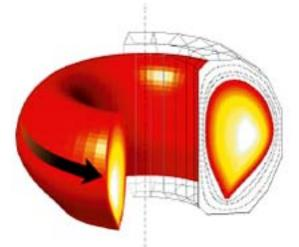
Figure 1: Artist's rendering of a tokamak plasma. The plasma is confined by the combination of strong magnetic field in the toroidal direction (around the hole in the "donut" as shown by the black arrow) generated by external coils (not shown) and the magnetic field from a large current flowing in the same toroidal direction. The plasma is held inside a sealed metal structure that is evacuated and lined with special material to keep the plasma pure and handle the heat exhaust.
