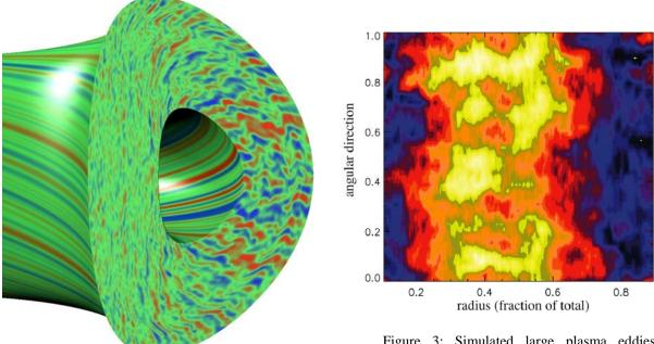
Figure 3: Simulated large plasma eddies excited by energetic fusion products.
