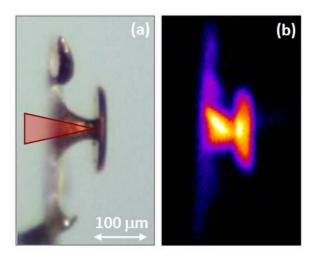
Figure 2: (a) Micro-scale Cu Flat-Top Cone target, with the incident laser (represented in red) coming from the left, (b) Cu K-alpha X-ray image showing the deep penetration of the laser light inside the cone neck.
