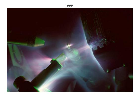
Figure 1: Image of the infrared laser (not seen, entering from left-hand side) interacting with a flat target (center), and the associated plasma production from the interaction on the various diagnostic instruments in the chamber. This is a time integrated image over five seconds. (Photo Credit: Joe Cowan and Kirk Flippo, LANL)
