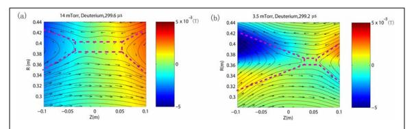
Fig.2; Comparison of neutral sheet configuration described by measured magnetic field vectors and flux counters for high (collisional) and low density cases; (a) Collisional regime ( $\lambda_{mfp} \sim 1 \text{mm} << \delta$ )); (b) Nearly collisionless regime ( $\lambda_{mfp} \sim 1 \text{cm} \sim \delta$ ). Out-of plane fields are depicted by the color codes ranged -50 G <Bt <50 G.
