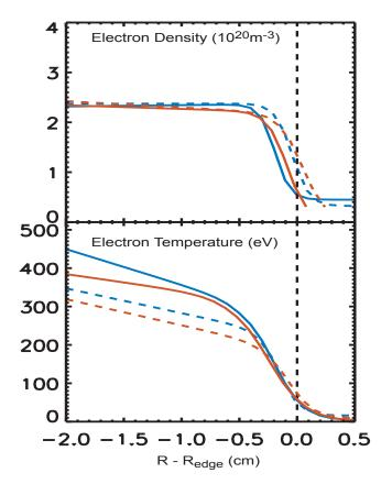
Sample plasma density and temperature pedestals with (dashed curves) and without (solid curves) additional gas puff. Density pedestal height remains fixed despite perturbation to neutral source.
