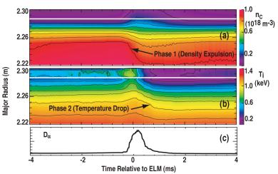
Fig. 2: Time and space evolution of (a) density of carbon ions and (b) ion temperature deduced from spectroscopic measurements on DIII-D. The white line in (a) and (b) indicates the outer boundary of the confined region. The deuterium light signal, which is indicative of the ELM timing, is shown in (c).
