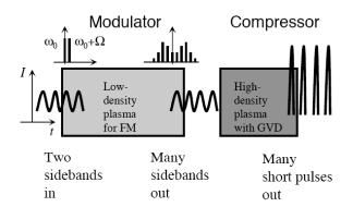
Schematic of the two-stage cascade compressor. Frequency modulation (FM) occurs in a rarefied plasma, after which the laser sidebands are compressed by means of the large group velocity dispersion (GVD) in a high-density plasma into a train of femtosecond spikes.
