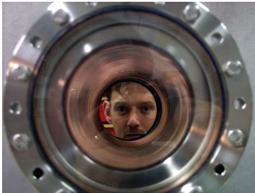
Figure 3. The initial field-reversed configuration (FRC) target plasma is formed inside a small (10-cm-diam) quartz tube. One of our AFRL collaborators, Chris Grabowski, provides the scale for the target plasma by looking through the tube.
