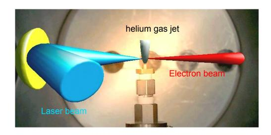
The laser beam is focused on the target. During its propagation, the gas is instantaneously transformed in an underdense plasma in which plasmas waves are excited. After breaking of these plasma waves electron beams are produced. Proton beams can be produced by replacing the gas jet with a thin foil target using the same experimental set-up. Note the very small size of the interaction zone.
