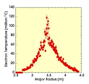
High electron temperature exceeding 100 million degrees Celsius is achieved in centrally focused microwave plasmas. It is observed a centrally peaked profile with a steep gradient, which suggests the suppression of the electron heat loss.
