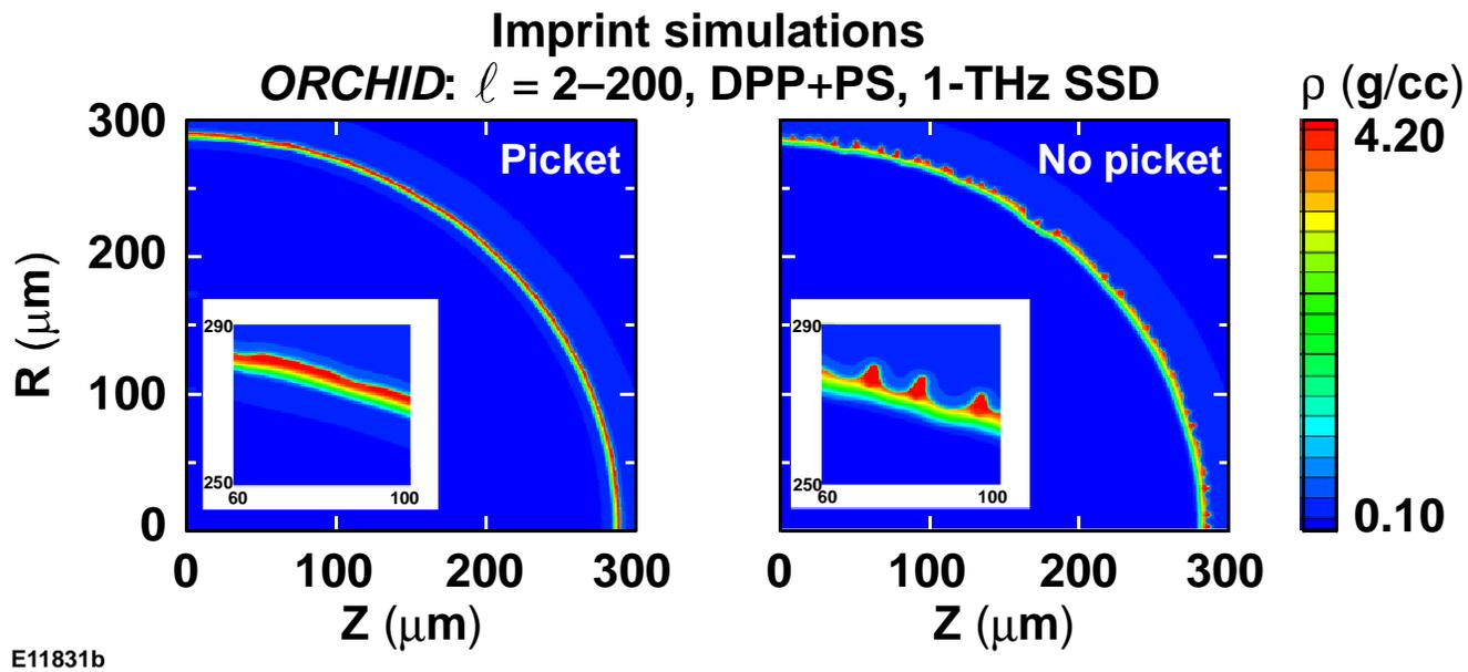
Target designer figure: Two dimensional ORCHID simulations showing the reduction in imprint-seeded modulations with a picket pulse
