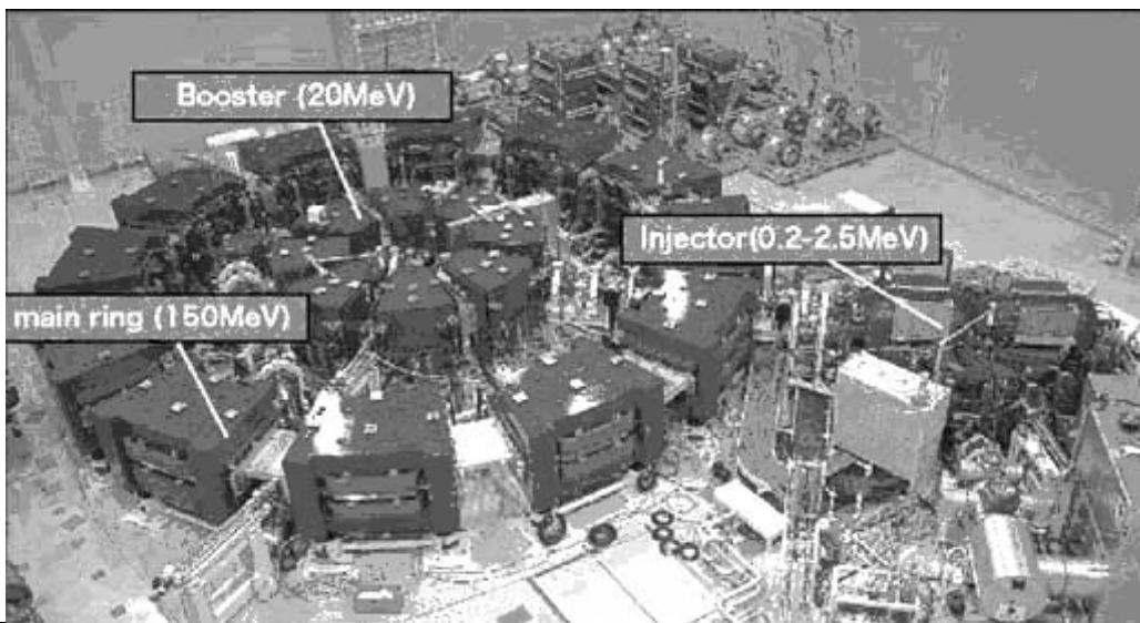
Figure 1. The three proton rings for ADSR studies at Kyoto Univ Research Reactor Institute in 2006.
