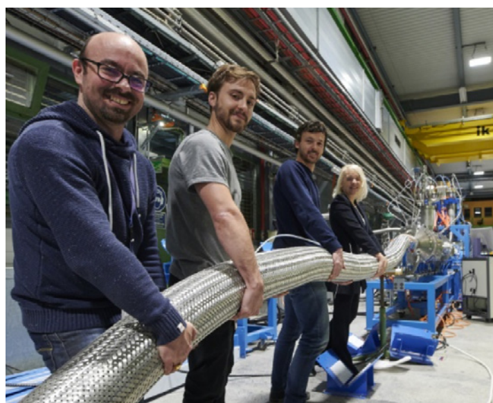
Figure 4. MgB 2 60-meter-long superconducting line with team members at CERN.
