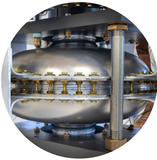
Image: Experimental setup for successfully demonstrating the conduction-linked cooling of a single SRF cavity. See page 22 for details. Photo Credit: Marty Murphy
