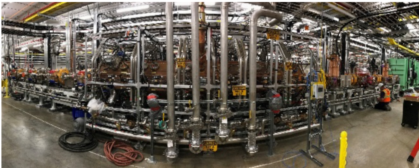
Figure 3. Aerial view of the room temperature lower LEBT including the 80.5 MHz RFQ during the front-end beam commissioning (ARR1) in 2017. The downstream SRF section is to the right.
