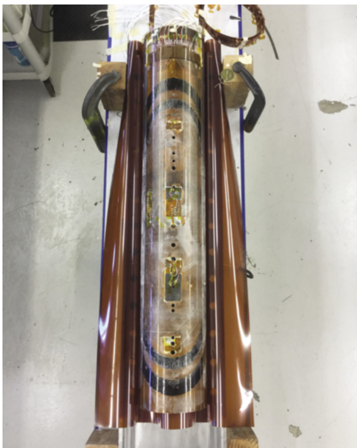
Figure 1. Image of the outer layer of the Cos( \theta ) magnet. The windings, end spacers and pole are visible, as are the voltage tap and strain gauge diagnostics. Signals from the diagnostics are routed to the magnet ends on a special “trace,” composed of lithography-processed copper on a kapton sheet, that is overlaid on the magnet and vacuum impregnated with the coil.
