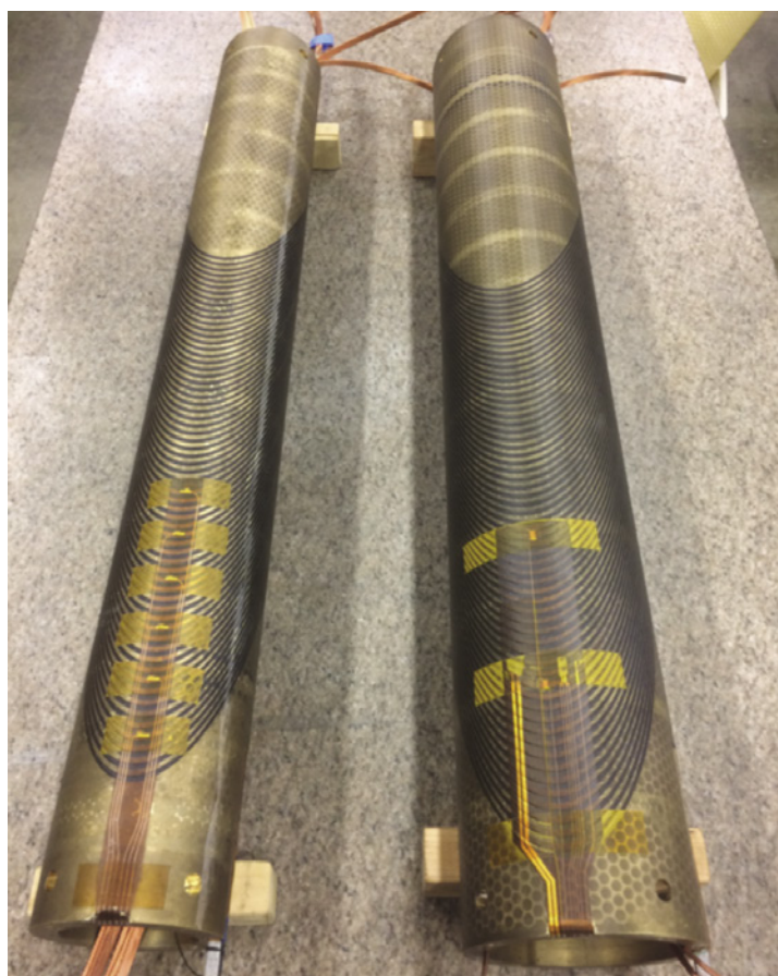
Figure 2. The two coils for the CCT5 magnet prior to assembly into the final magnet structure.
