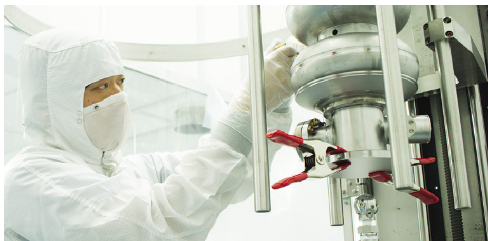
Figure 2. A researcher works on superconducting RF accelerating cavity at Cornell University. The quality of the interior surface of the cavity determines performance, and the Center for Bright Beams is studying the impact of doping, impurities and trapped magnetic flux.
