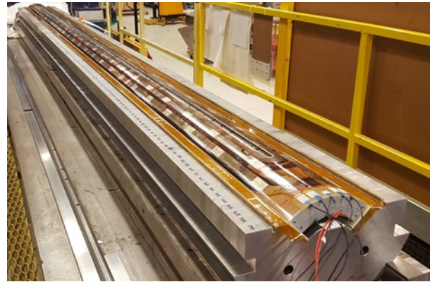
Fig. 4: Long MQXF coil being assembled in a mirror structure (credit: R. Bossert, F. Nobrega)
