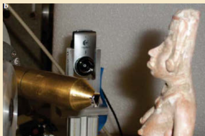
Figure 2: Figurine found in Mesoamerican burial grounds and currently housed at the University of Notre Dame's Snite Museum of Art. The figurine is mounted on the proton-induced X-ray emission (PIXE) beam line at Notre Dame's 11-MV electrostatic accelerator to obtain quantitative details of the pigment composition; in particular, PIXE reveals the iron and manganese content of the paint.
