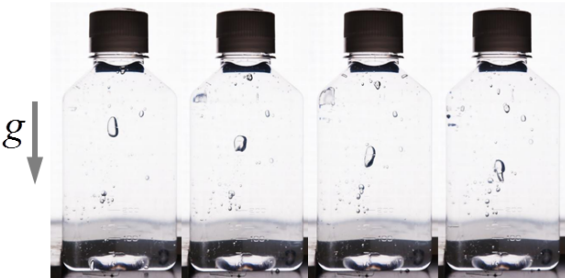
Time series of an air bubble forced to sink within a complex fluid. (Credit: University of Illinois at Urbana Champaign.)
