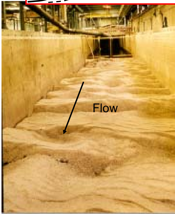
Dunes in a channel at St. Anthony Falls Laboratory, University of Minnesota, USA
