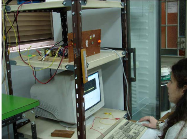
A researcher measuring very slow dielectric relaxation glucose glasses with equipment designed and constructed in Grigera's lab.
