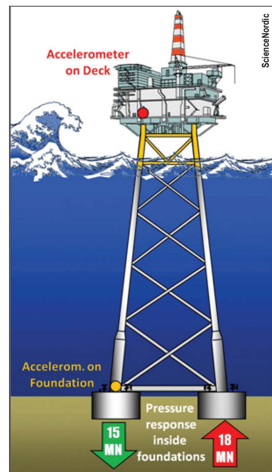
Measurements in 1995 with instruments on the Draupner oil-drilling rig confirmed a rogue wave height of 85 feet.
