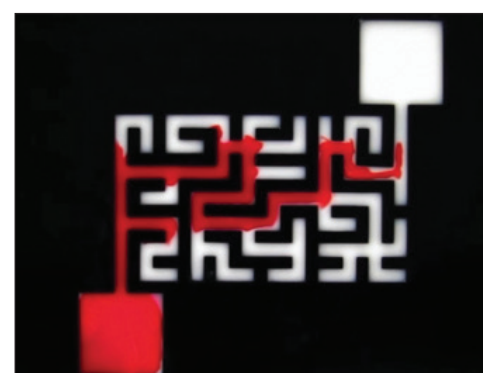
Soap Opera in the Maze (V0098): Thanks to surface tension, soap molecules can follow the correct path out of a labyrinth of channels. doi.org/10.1103/APS.DFD.2017.GFM.V0098
