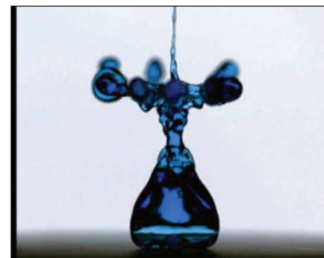
Kicking Droplets (V0080): Droplets on vertically moving plates form intricate shapes when they lift off. doi.org/10.1103/APS.DFD.2017.GFM.V0080
