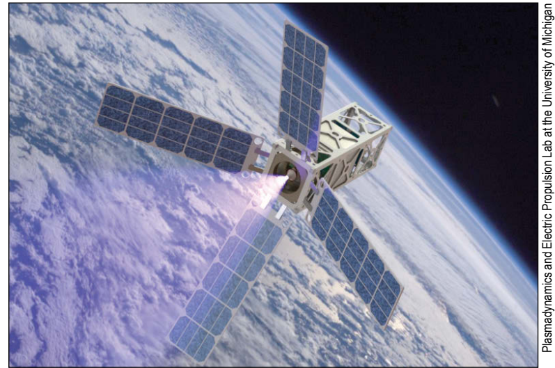
Small satellites called CubeSats can be steered and propelled by tiny ion and plasma thrusters.
