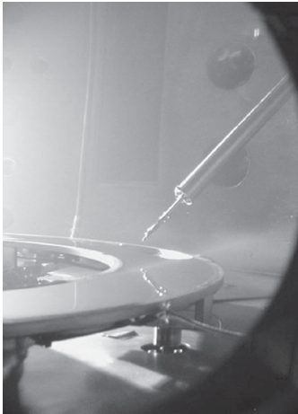
Pool of liquid lithium in the tray that encircles the bottom of the CDX-U device. The tip of the liquid-lithium injector, which is removed before plasma operations, is reflected on the shiny surface of the liquid lithium.
