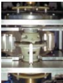
Rotating ring (center), roughly the diameter of a compact disk, cycles powdered magnetic material in and out of a gap in the powerful magnet at rear.
