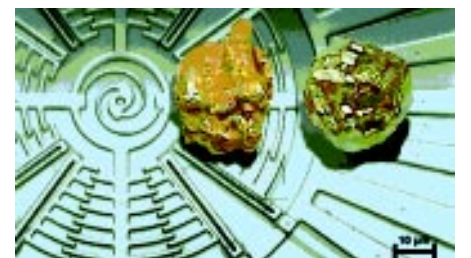
The background image is part of a 2-millimeter ‘rotor disk’ made out of polysilicon freely suspended in mid-air, only supported in the center by a 2-micron (!) ‘anchor post.’ The rotor is spun with electrostatic comb drive assemblies and optical modulators (right).
