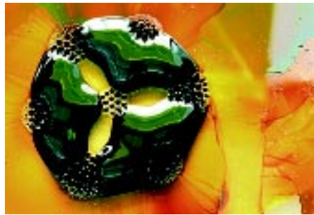
Ferrofluid on a glass surface, with 7 circular magnets. From On the Surface of Things, Images of the Extraordinary in Science by Felice Frankel and George M. Whitesides
