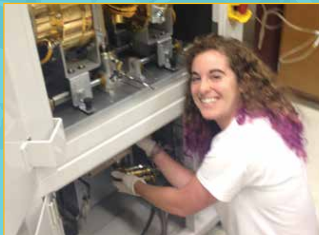
Eliza Cohn , a Charlottesville high school student worked in the lab of Despina Louca in the department of Physics at the University of Virginia. She is preparing a floating zone furnace used to grow single crystals for condensed matter research. Eliza is now a student at Johns Hopkins University.
