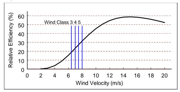
**Figure 3**. % rated power of 600 kW wind turbine for wind strength classes 3, 4 and 5 for wind turbine curve shown in Figure 2A (See Table 1). The horizontal axis is the *average* wind velocity at a given site assuming a Rayleigh distribution of wind velocity values.
