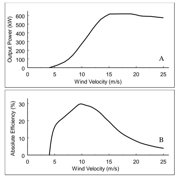
**Figure 2.** A) Power output for a 600 kW wind turbine. (Data digitized from [5], "The Power Curve of a Wind Turbine") B) Absolute efficiency of 600 kW wind turbine: power output (graph A) divided by total power in moving air mass.
