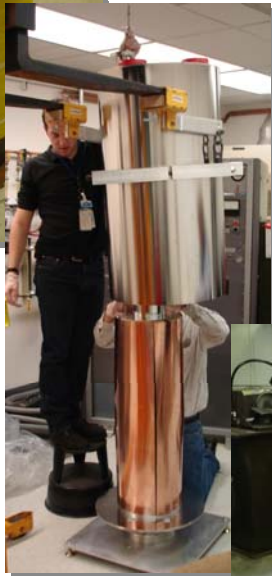
Field compensation magnet for SQUIDs
