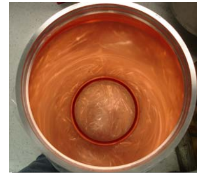
New microwave cavity
