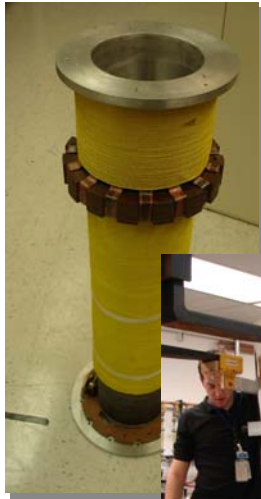
Field compensation magnet for SQUIDs
