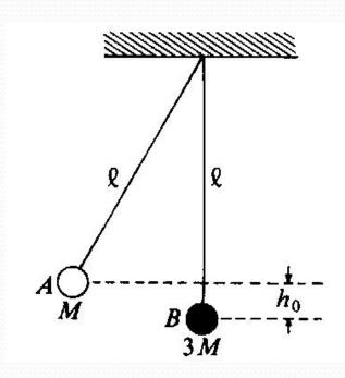
5. Two small spheres of putty, A and B, of mass M and B, respectively, hang from the ceiling on strings of equal length  $\ell$ . Sphere A is drawn aside so that it is raised to a height  $h_0$  as shown above and then released. Sphere A collides with sphere B; they stick together and swing to a maximum height h equal to
